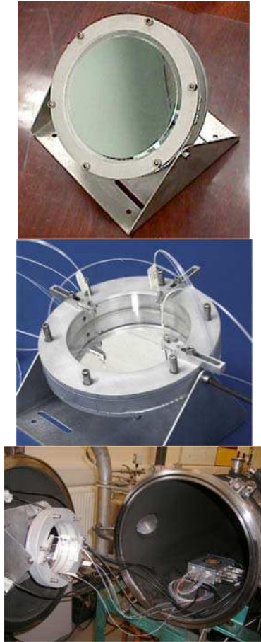
Figure 4. The front (top) and back (middle) views of a prototype FOMIS unit. The bottom image shows the unit and the electronics inside the two-stage light gas gun test chamber at Kent. Right before the closing of the chamber, the unit was turned 180° to allow the front side to face the incoming projectile.
