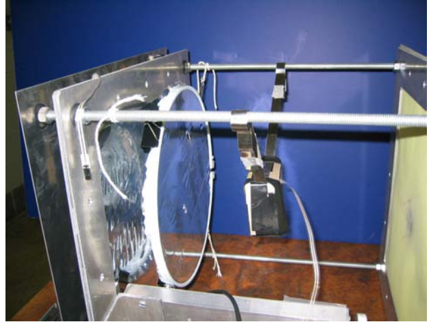
Figure 2. One of the configurations of the test. The square target film (to the left) had an exposure area of 30 cm by 30 cm while the second target hoop had a diameter of 26 cm. Two PVDF sensors were attached to each film while a third one was attached to the frame. A hanging piece of aerogel was also used as the third target.
