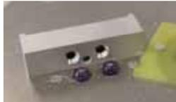
Figure 6. APD assembly mounted on target plate
