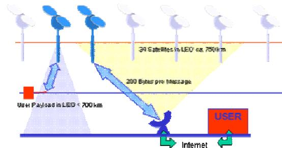
Figure 3. MDD-experiment data transmission concept
