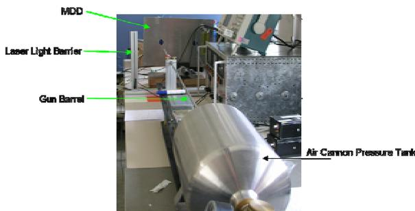
Figure 9. Air Cannon Test Setup
