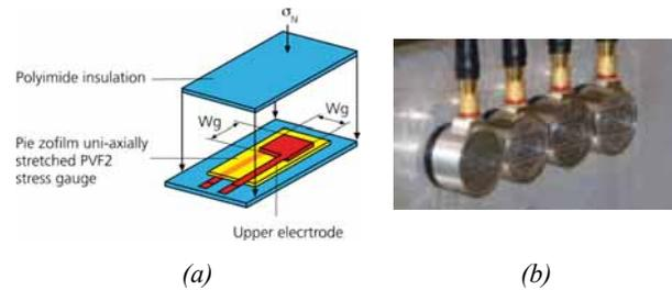
Figure 4. (a) PVDF stress gauge representation (b) ultrasonic transducers
