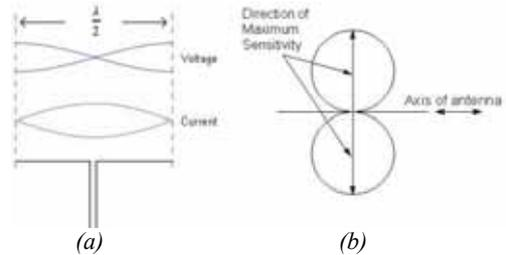
Figure 8. Dipole antenna characteristics (a) current and voltage distribution pattern, (b) horizontal polar diagram
