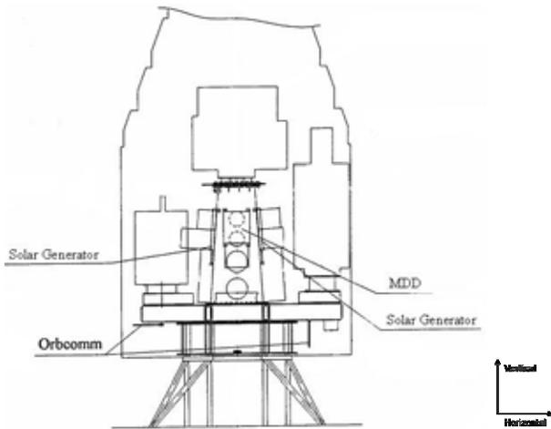
Figure 2. MDD integration onto Cosmos Upper stage
