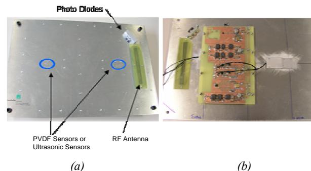
Figure 1. Photo of MDD (a) top side of target plate with Photo diode and antenna assemblies (b) rear side of detector plate with electronics
