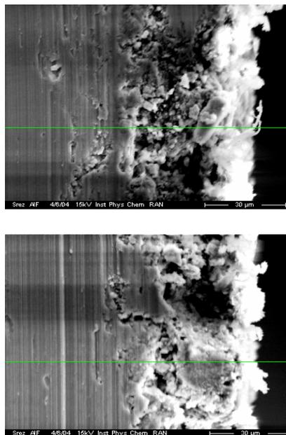
Figure 4. Electron microscopic image of the transversal microsection surface (over:  $v \approx 300$  m/s,  $\gamma \approx 7^{\circ}$ ; below:  $v \approx 450$  m/s,  $\gamma \approx 11^{\circ}$ )
