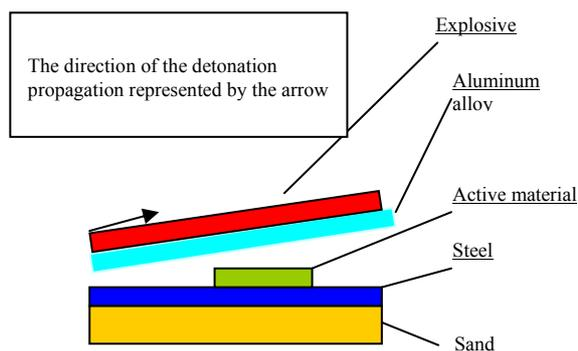
Figure 2. The shock loading scheme
