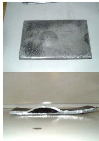
Figure 3. Appearance of assembly after impact and section of assembly on a median plane (polythene – over, teflon – below;  $v = 300 \text{ m/s}$ ,  $\gamma \approx 7^\circ$ )
