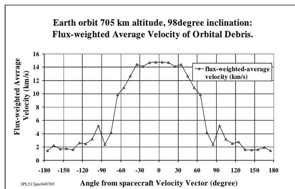
Figure 4. Average velocity of OD impact, as a function of angle measured from the spacecraft velocity vector, for the stated orbit.
