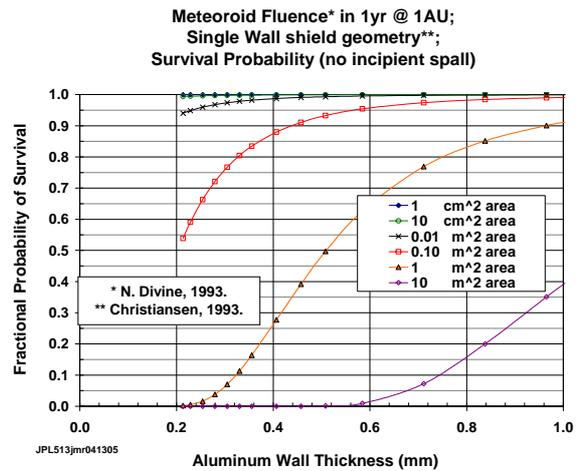
Figure 1. Survival probability of a single-wall M/OD shield in a 1 AU heliocentric orbit for 1 year. Average surface fluence and normal-incidence impact are assumed.
