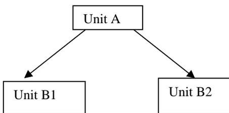
Figure 5. Diagram of redundant units B1 and B2 that are both controlled by a third unit A that has no redundant counterpart.
