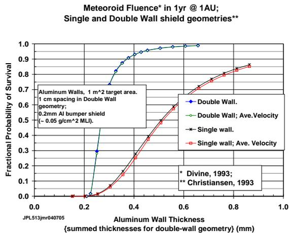
Figure 3. Survival probability of a 1m<sup>2</sup> target in the 1AU meteoroid environment for 1 year. Double- and Single-Wall target geometries are shown. Calculations use either an environment binned in 1 km/s velocity increments, or use the particle-fluence-weighted average velocity of 16 km/s. Average surface fluence and normal-incidence impact are assumed.
