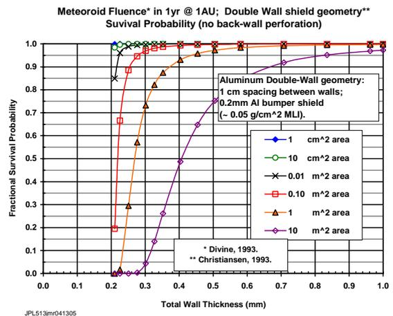
Figure 2. Survival probability of a double-wall M/OD shield in a 1 AU heliocentric orbit for 1 year. Average surface fluence and normal-incidence impact are assumed.
