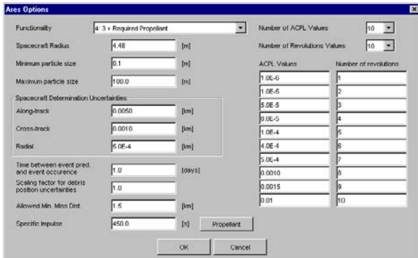
Figure 3. An example of the user input (for ARES) provided by the DRAMA GUI.
