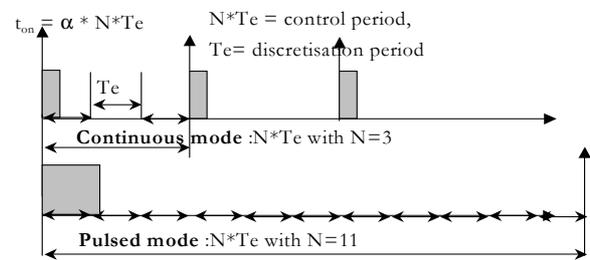
Figure 9. Thrust modes, continuous and pulsed
