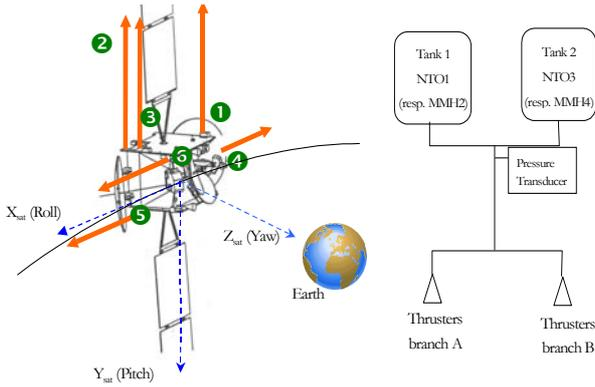
Figure 6. (left) satellite in Earth-pointed attitude, (right) liquid feedlines for a pair of tanks (NTOx or MMHy)
