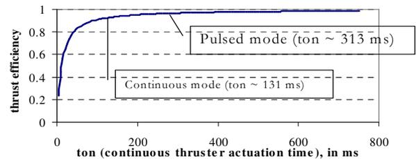
Figure 10. Thrust efficiency as function of actuation time
