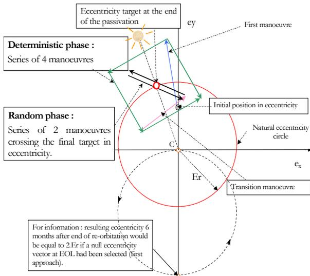
Figure 7. Manoeuvre sequence and strategy for control in eccentricity
