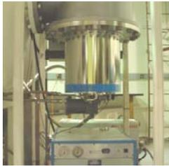
Figure 12: Oil-free He cryopump
