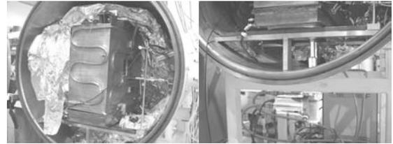
Figure 9: LN<sub>2</sub> enclosure and Cryogenic refrigerator
