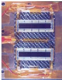
Figure 13: Electrically biased solar cell setup
