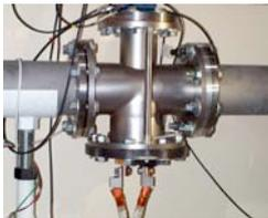
Figure 4: Magneforming shutter
