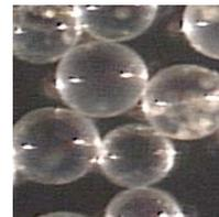
Figure 6: Soda lime glass particles
