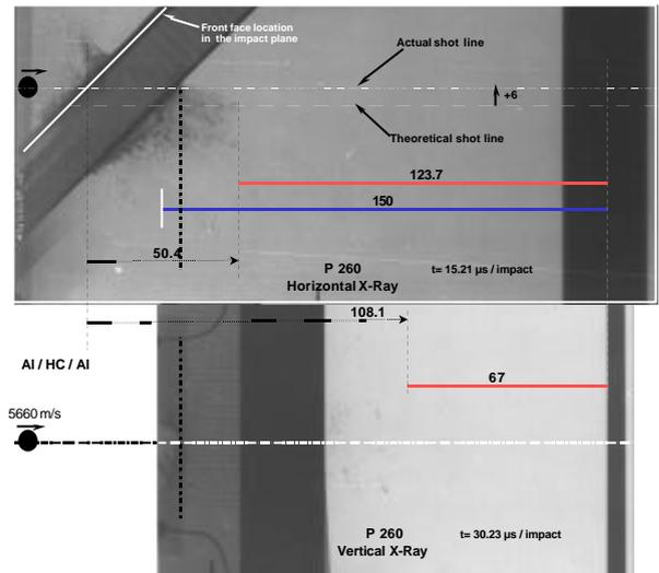
Fig. 7. Flash X-Ray radiographs taken during shot #P260. Honeycomb structure with aluminium facesheets.
