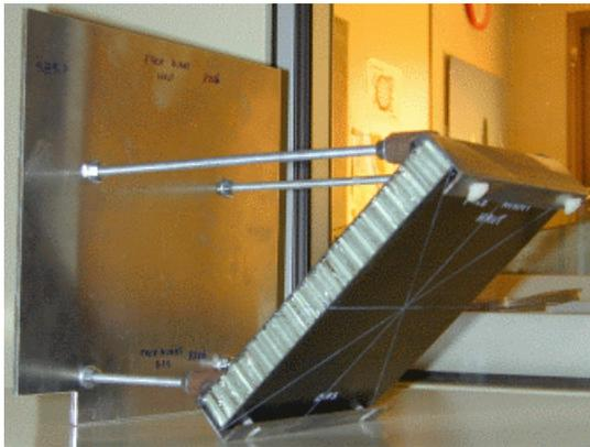
Fig. 2. : target assembly at 45° incidence.
