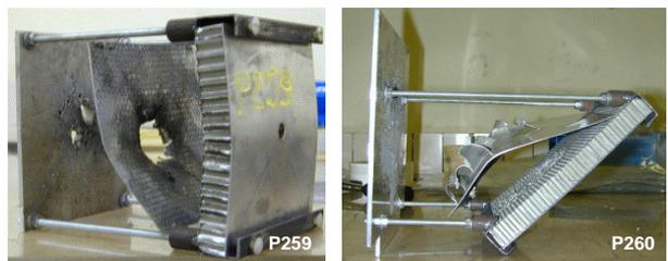
Fig. 9. Post shot targets. Aluminium facesheets panels at normal and 45° incidence.
