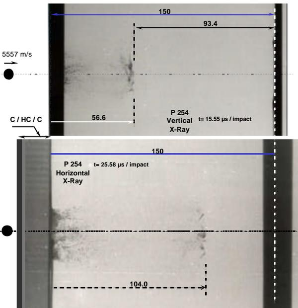
Fig. 6. Flash X-Ray radiographs taken during shot #P254. Honeycomb structure with carbon composite facesheets.
