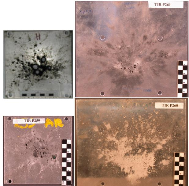
Fig. 12. Witness plates as seen from projectile – left: normal incidence; right: 45° incidence; top: carbone composite facesheets; bottom: aluminium facesheets.
