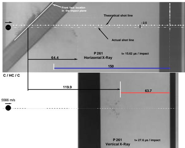
Fig. 8. Flash X-Ray radiographs taken during shot #P261. Honeycomb structure with carbon composite facesheets.
