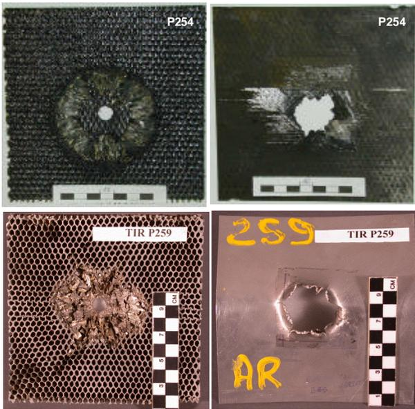
Fig. 10. Honeycomb structure and rear facesheet damage at normal impact incidence as viewed from the witness plate– Top: carbon composite facesheets; bottom: aluminium facesheets.
