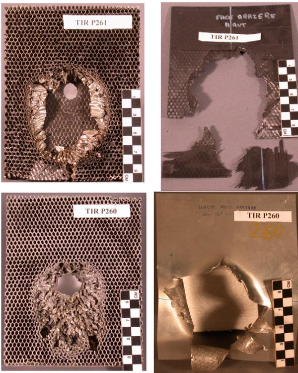
Fig. 11. Honeycomb structure and rear facesheet damage at 45° impact incidence as viewed from the witness plate – Top: carbon composite facesheets; bottom: aluminium facesheets.
