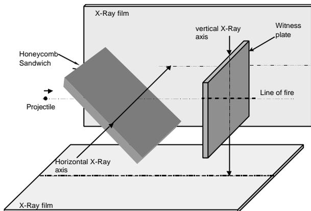
Fig. 3. Sketch of experimental configurations at the gun muzzle (shown here at 45°).
