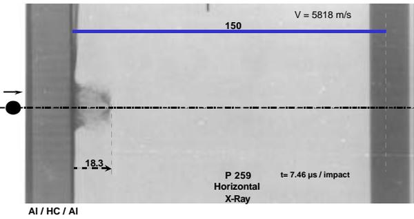
Fig. 5. Flash X-Ray radiograph taken during shot #P259. Honeycomb structure with aluminium facesheets.
