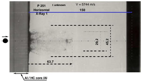
Fig. 4. Flash X-Ray radiograph taken during shot #P251. Honeycomb structure with aluminium facesheets.
