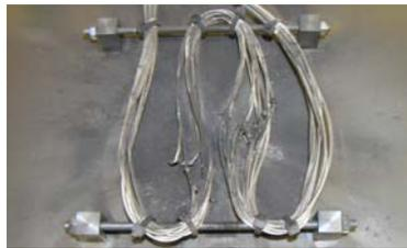
From the electrical measurements made during impact (Fig. 13), the potential difference between the cables operating at 28 V and those operating at 50 V was determined. This voltage should be constant if there is no conducting bridge between the circuits. Simultaneously, an electrical current flowing from one circuit into the other was measured, peaking at about 9 A. This indicates that the conductors from both circuits were in temporary contact during impact (ca.
