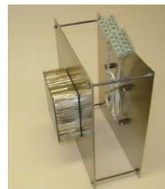
Figure 10. Complete target showing RAD1 CFRP H/C SP mounted on a frame holder and harness mounted on the witness plate
