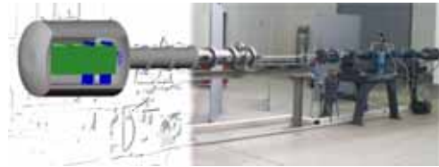
Fig.2 Two stage light gas gun ( Pictured by CISAS)
