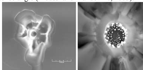
Figure 3 Normal HVI of iron dust on glass. On the right, a picture of the pit observed on glass at very high velocities showing evidence of Fe residue droplets
