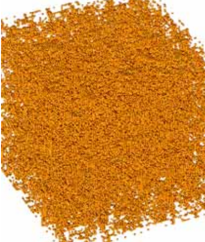
Figure 6. An open-cell foam, whose weight is 9.2% the weight of solid Aluminum, is created by the program, and showed as SPH particles.
