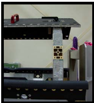
Figure 3. Picture of the connection between floor and side panels.
