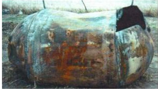
Figure 5. Photograph of reentered Delta II Stage II tank showing apparent molten hole (photo courtesy NASA).
