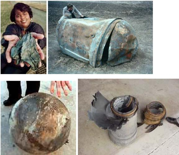
Figure 2. Debris from Delta II Second Stage reentry: clockwise from top left: Lightweight fragment, propellant tank, thrust chamber, sphere. Photos courtesy Tulsa World (staff photo by Brandi Stafford), NASA, Aerojet, NASA, respectively.
