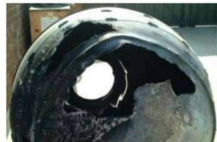
Figure 8. Photograph of reentered Delta Third Stage tank showing molten holes.
