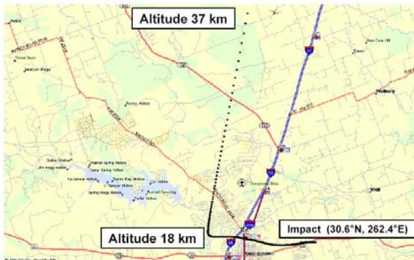
Figure 3. Best-estimate trajectory for the propellant tank.
