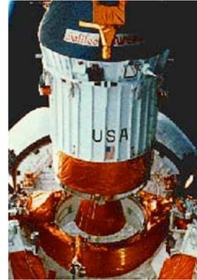
Figure 1: Picture of an IUS with both stages in the space shuttle bay (courtesy of NASA)
