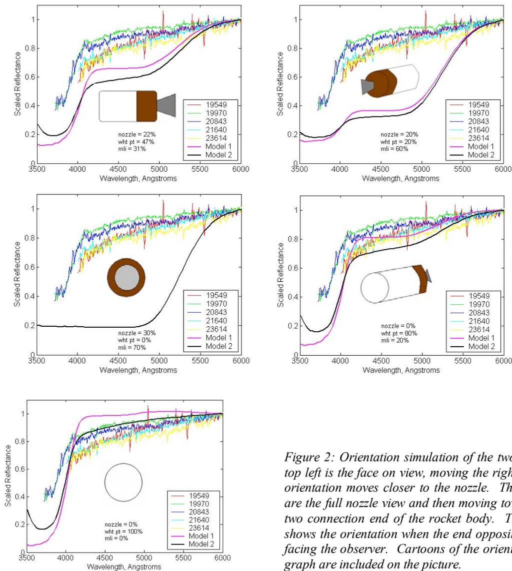
Figure 2: Orientation simulation of the two models. The top left is the face on view, moving the right shows as the orientation moves closer to the nozzle. The middle rows are the full nozzle view and then moving toward the stage two connection end of the rocket body. The final figure shows the orientation when the end opposite the nozzle is facing the observer. Cartoons of the orientation for each graph are included on the picture.
