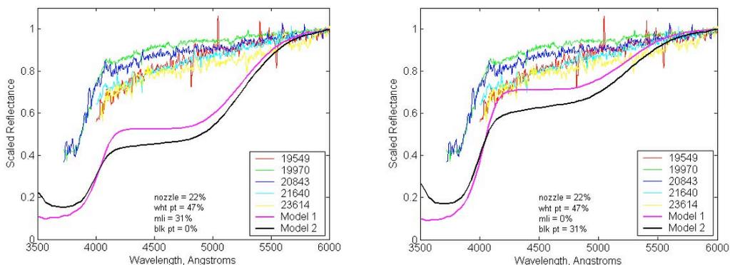
Figure 3: Models of MLI presence on the nozzle of the IUS. Model 1 uses pristine material and model 2 uses flown white paint. The figure on the left shows what the spectrum would look like if the MLI was still on the nozzle and covering the solid rocket motor. The figure on the right depicts the spectrum if the MLI on the solid rocket motor was not visible (or no longer there) but still remained on the nozzle. No evidence of the MLI is seen in the remote samples.
