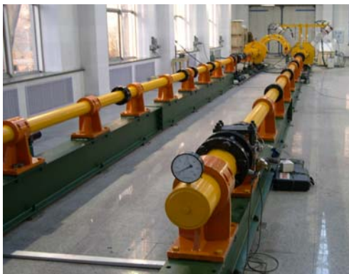
Fig.1 Setup of Two-state light gas gun Fig.2 Layout of Acoustic Emission sensors
