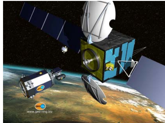
Figure 5. A UA carrying an EM is approaching a client satellite supervised by an EA.
