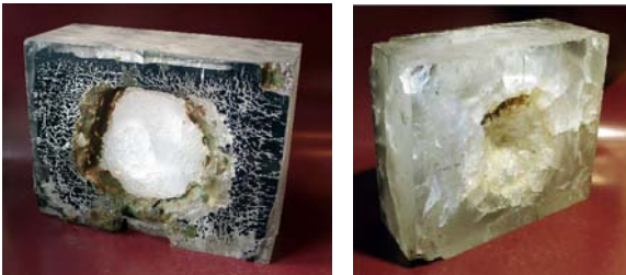
Figure 7. Craters in the thick PMMA plate after impact of the 1 g solid with velocity of \sim 6 km/s.
