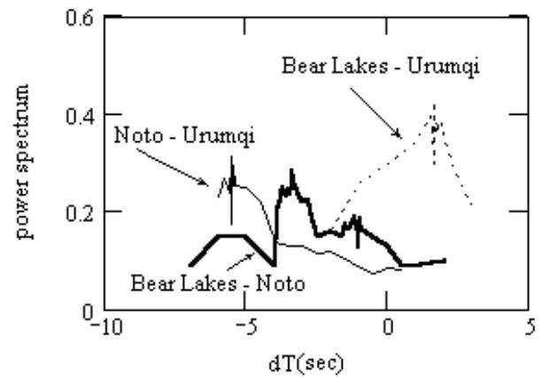
Figure 7. Time dependence of cross-spectrum maximums of Cosmos-1366 at baselines Bear Lakes-Noto, Bear Lakes-Urumqi and Noto-Urumqi.
