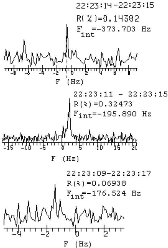
Figure 5. The cross-spectrum of echo from Cosmos-1366, at baseline Bear Lakes-Noto, Urumqi-Noto and Bear Lakes-Urumqi. Fringe rates are measured as frequency of spectral maximums:  $-373.703$  Hz,  $-176.524$  Hz and  $-195.890$  Hz respectively. VLBR03.1.
