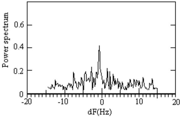
Figure 3. The TA-RA cross-spectrum Evpatoria-Urumqi baseline, for Raduga-9. Doppler shift evaluated as frequency of spectral maximum is 1574.147 Hz, frequency resolution is 0.234 Hz, VLBR03.1.
