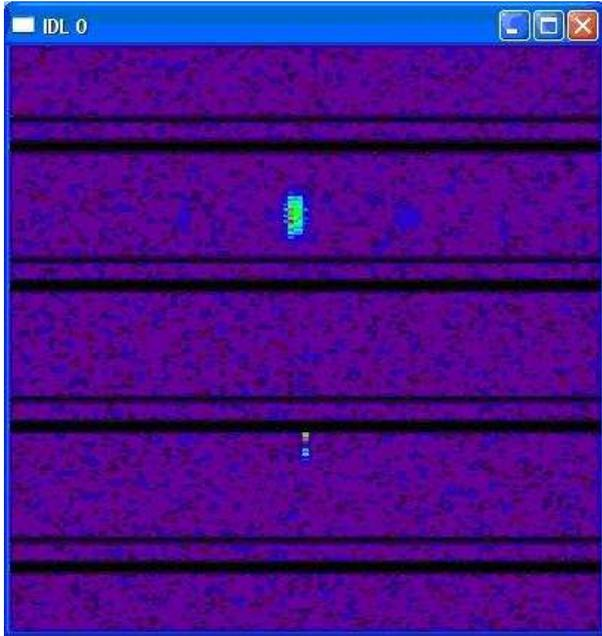
Figure 8. The sample of frequency-time diagram for analyzing the beam-track experiments. The vertical axis is time from 22:12:31 to 22:16:41 of day 206, 2004. The horizontal line is frequencies 247802.734 262451.172. The two points are identified with COSMOS 1961 and TELESAT-5.
