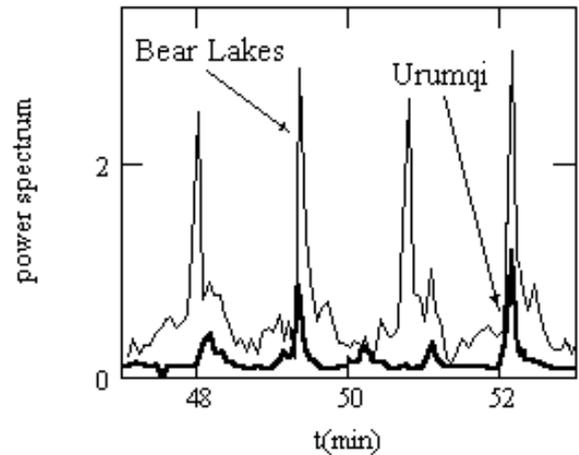
Figure 4. Dependence of spectral maximum on time (TA-RA cross-spectra for Raduga-9 on Evpatoria-Bear Lakes and Evpatoria-Urumqi baselines), time resolution is 4.26 s, real period of rotation is 166 s.
