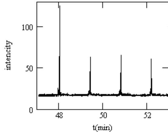
Figure 2. Recording of echo intensity of Raduga 9, estimated period of rotation is 83 s.
