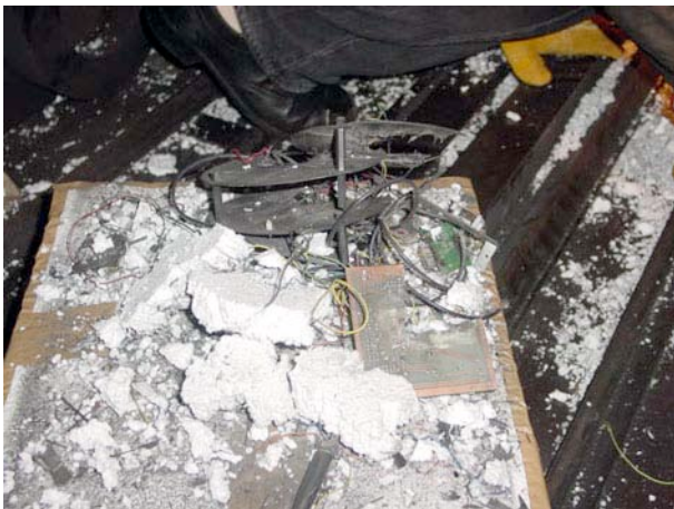
Figure 4. Micro satellite fragmented after low-velocity impact.
