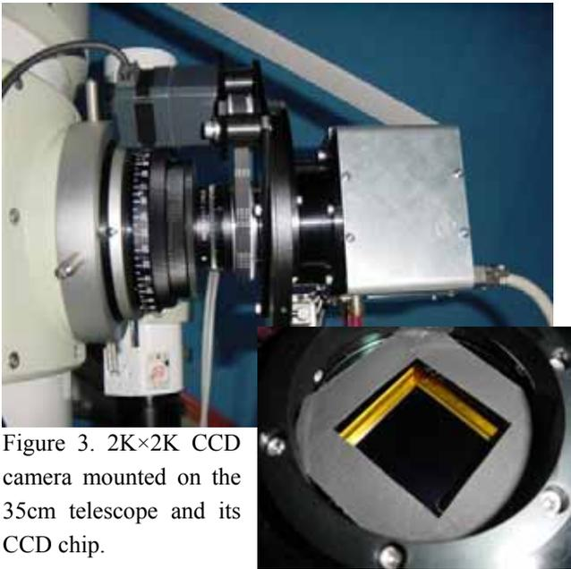
Figure 3. 2K×2K CCD camera mounted on the 35cm telescope and its CCD chip.
