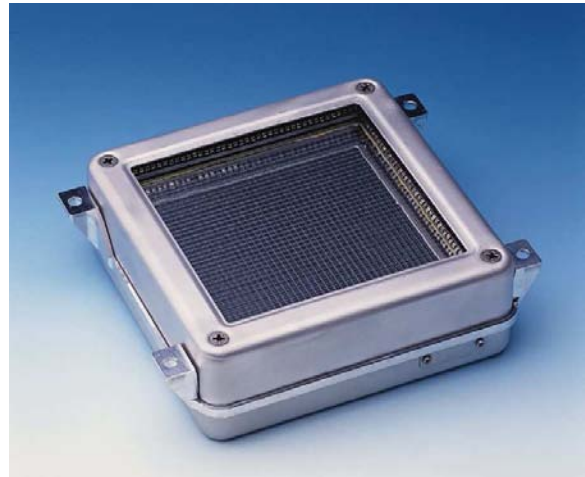
Figure 1. A DEBIE Sensor Unit Flight Model.
