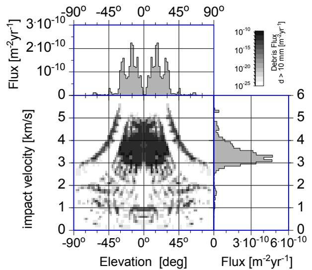
Fig. 9: Debris flux (fragments only) for  $d > 1\text{cm}$  on a GEO target as a function of impact elevation angle and impact velocity (SA)
