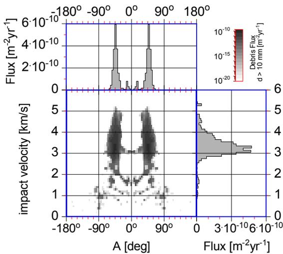
Fig. 8: Debris flux (fragments only) for  $d > 1\text{cm}$  on a GEO target as a function of impact azimuth angle A and impact velocity (SA)
