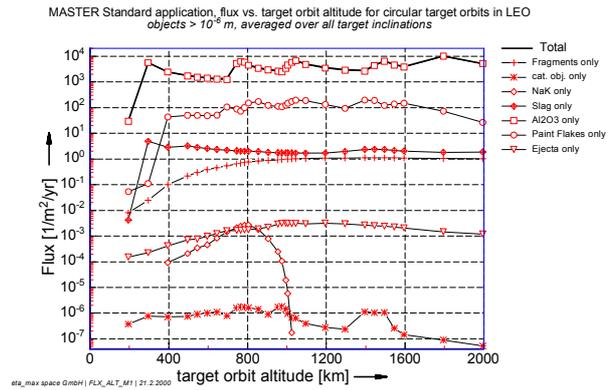
Figure 6 Flux resulting from objects larger than 1micron vs. (circular) target orbit altitude. (averaged over all inclinations) (SA)
