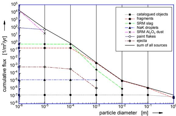
Figure 5 Flux vs. size resulting from different sources for an ISS like orbit ( $i=50,5^\circ$ ,  $h=400$  km) (SA)
