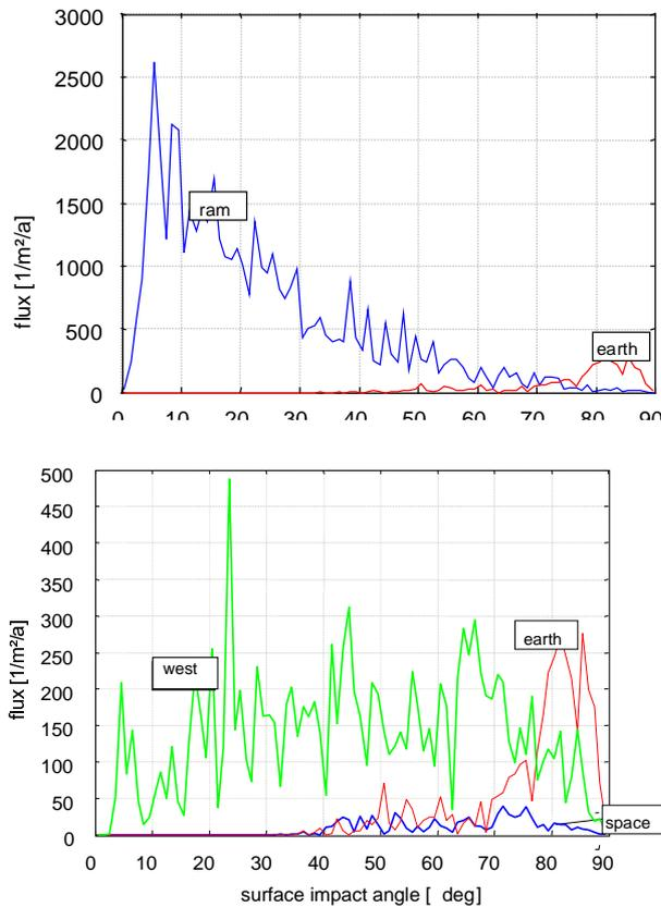
Fig. 11: Surface impact angle distribution of the debris flux > 1 μm on an ERS like satellite (earth oriented target)
