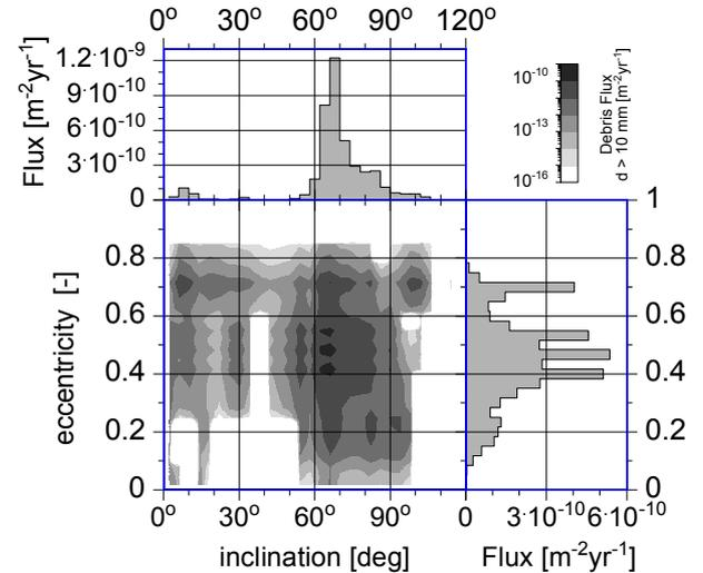
Fig. 7: Debris flux (fragments only) for  $d > 1$ cm on a GEO target as a function of particle eccentricity and particle inclination (SA)
