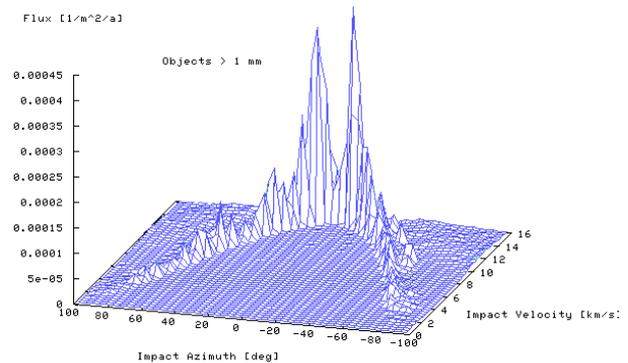
Fig. 10: Flux distribution vs. impact azimuth and impact velocity for a sun-synchronous ERS like target
