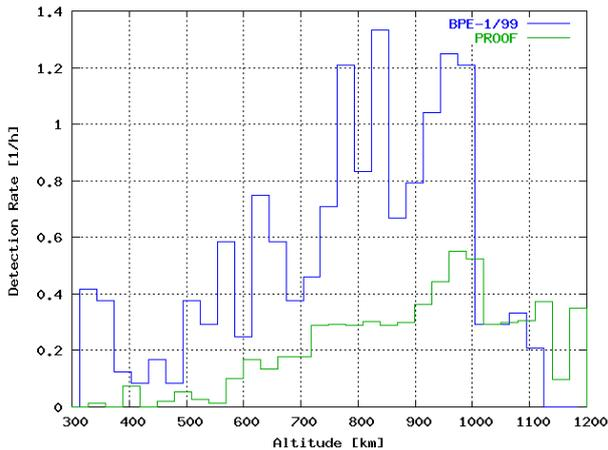
Fig. 3. Altitude Spectrum of the BPE-1/99 experiment compared to PROOF prediction
