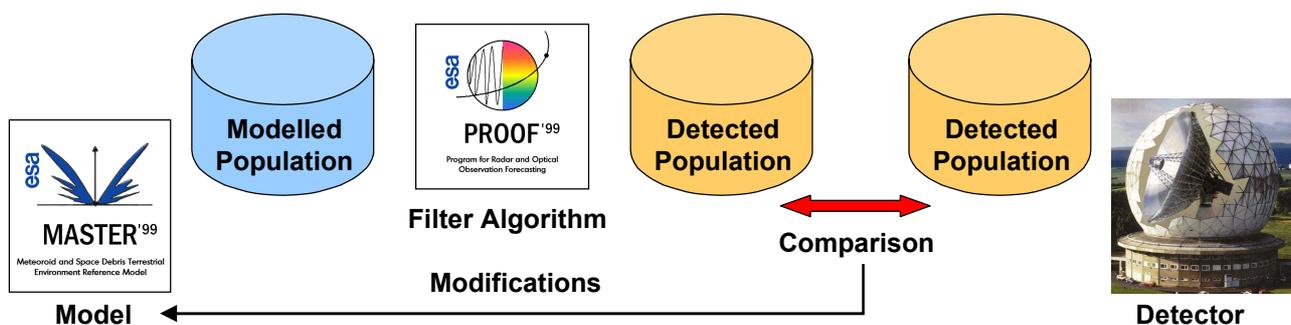
Fig. 1. Processing scheme for comparisons between space debris models and detector results
