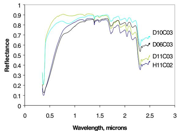
Fig. 3. White Paint on the Clamps on LDEF.
