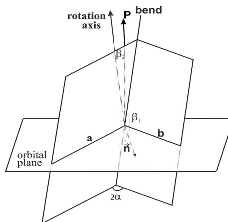
Fig.1. The model of the space debris fragment.
