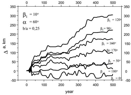
Fig.2. The 500-year evolution of semimajor axis of near GEO debris particle.
