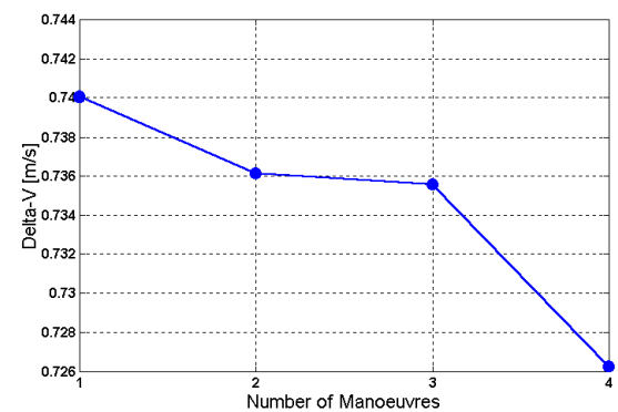
Fig. 8. Delta-V as function of the number of performed thrust arcs (or manoeuvres)
