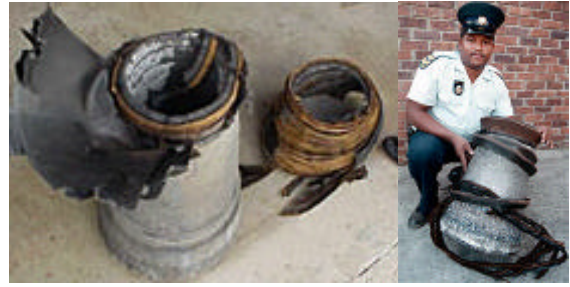
Fig. 8. Comparative image of the DELTA II second stage thrust chamber that impacted in Texas on the left, and thrust chamber that impacted near Robertson in the western Cape on the right. Similarities are obvious
