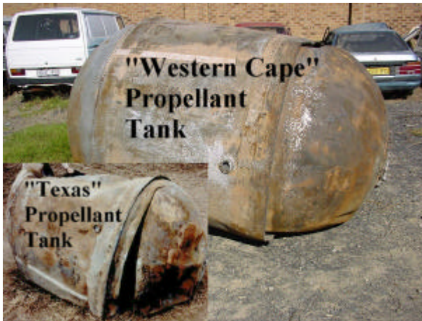
Fig. 6. Composite image of the propellant tank that impacted near Durbanville in the western Cape and the DELTA II second stage propellant tank that impacted in Texas on 22 January 1997. Similarities are obvious.
