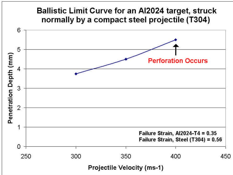
Figure 5 Results of the validation simulations to determine the accuracy of the element failure strains. They are found to be in good agreement with empirical perforation data.
