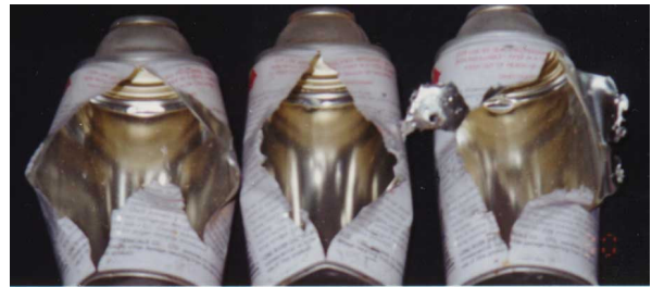
Fig.3 Damage of Water and Gas Filled Can Impacted at The Site under The Water
