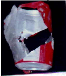
(b) Rear-Wall Catastrophic Rupture
