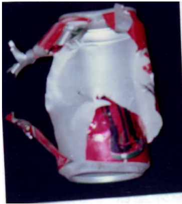
Fig.7 Rear Wall Catastrophic Rupture Of Pressurized Can
