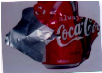
(a) Front-Wall Catastrophic Rupture
