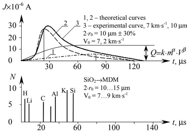
Fig.2. Spectral and integral dependencies of current pulse
