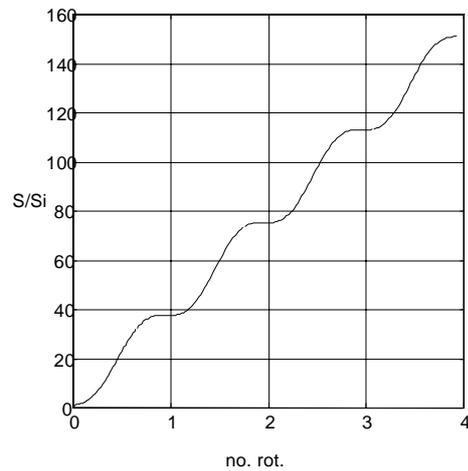
Fig. 1 Relative length variation of the tether (without strenght)
