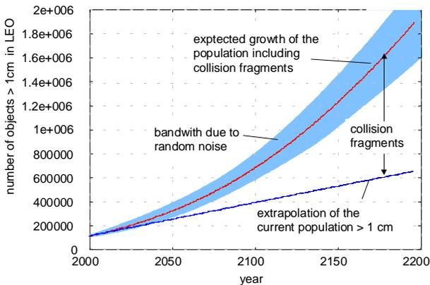
Fig. 2. The principle growth of the future debris population > 1 cm in LEO without any debris mitigation
