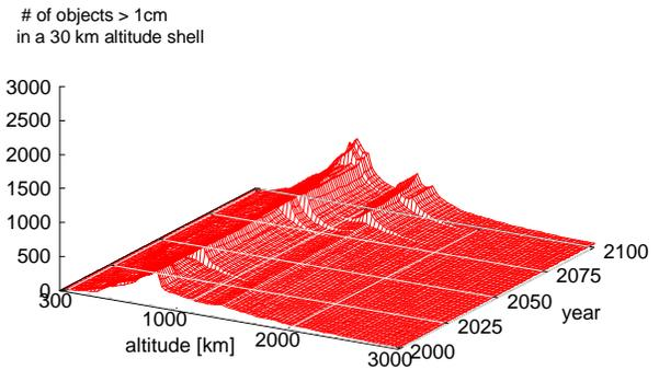
Fig. 7. Example for future debris population > 1 cm in LEO, immediate de-orbit and explosion prevention
