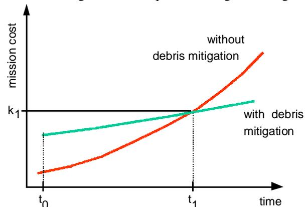
Fig. 1. Principle cost net benefit of debris mitigation due to mitigation implementation time
