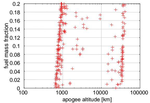
Fig. 10 Propellant mass fractions required to reduce the orbital lifetime according to Fig. 8
