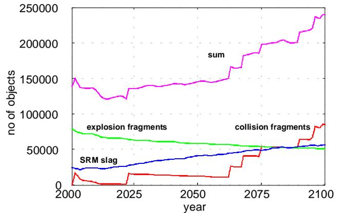
Fig. 8. Example for the future debris population > 1 cm in LEO, immediate de-orbit and explosion prevention
