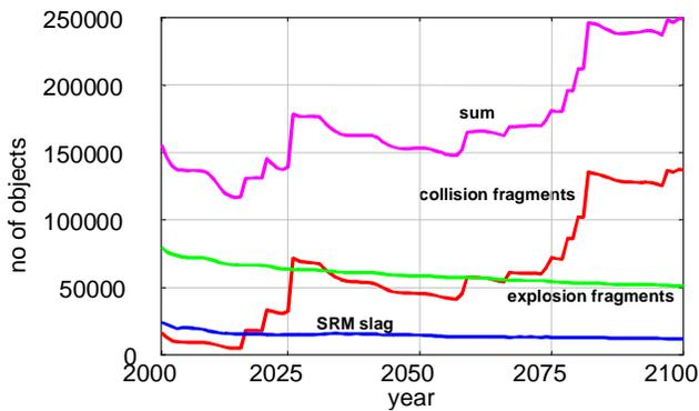
Fig. 12. Example for the future debris population > 1 cm in LEO, immediate explosion and SRM slag prevention
