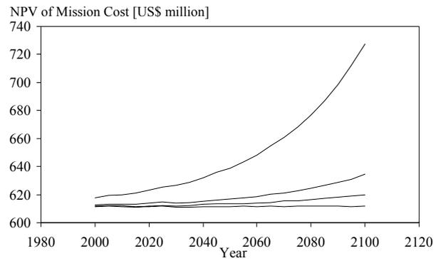
**Fig. 2.** Net present value of an Orbcomm-type mission with year initiated, for mitigation scenario S1. From top to bottom: 1-mm, 1.995-mm, 3.162-mm and 1-cm debris.
