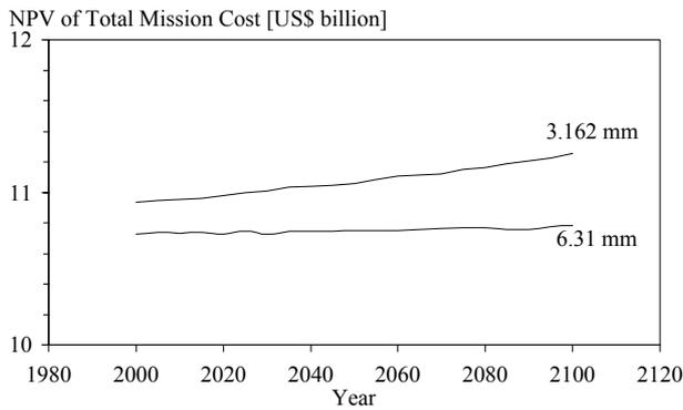
**Fig. 3.** Variation in the present value of the total mission cost of a Teledesic-type mission with year initiated, for 3.162-mm and 6.31-mm debris, for scenario S1, assuming that an impact with an object of each respective size will induce satellite failure.
