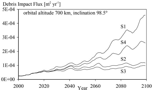
**Fig. 1.** 1-cm debris growth from 2000 to 2099 for an example orbit, as determined by EVOLVE, for the four different scenarios specified in the text.
