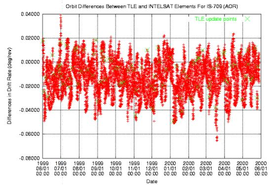
**Fig. 3a.** Orbit differences between TLE and INTELSAT elements in orbital frame for IS-709 (AOR).
