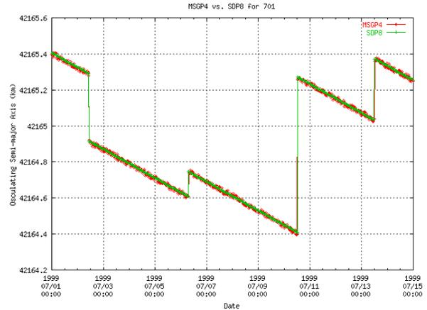
**Fig. 2a.** Comparisons of semi-major axis between SDP8 and MSGP4
