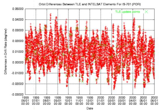
**Fig. 4a.** Orbit differences between TLE and INTELSAT elements in orbital frame for IS-701 (POR).
