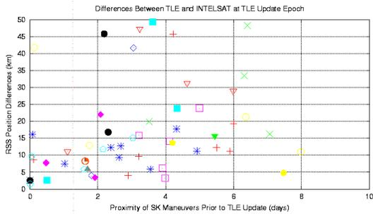
**Fig. 8.** Effects of station-keeping maneuvers on the accuracy of TLE at TLE update epoch.
