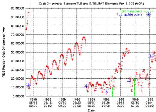
**Fig. 7.** Effects of station-keeping maneuvers on the accuracy of TLE within TLE update cycles.
