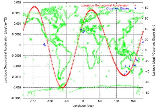
**Fig. 6.** Observed tangential biases as a function of geopotential acceleration.
