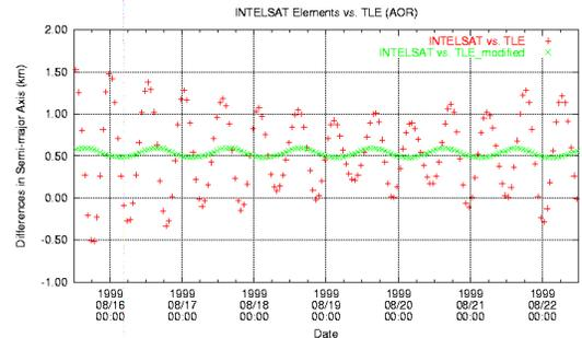
**Fig. 10.** Modified TLE comparisons with INTELSAT orbit.
