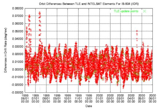
**Fig. 5a.** Orbit differences between TLE and INTELSAT elements in orbital frame for IS-804 (IOR).
