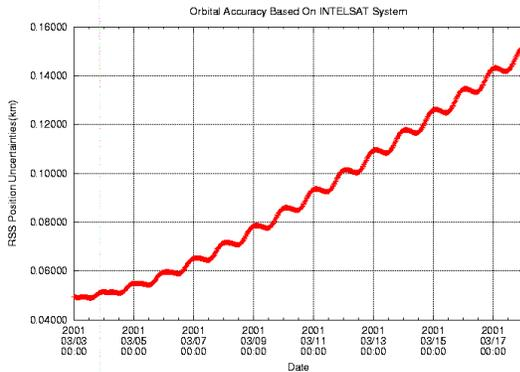
**Fig. 1.** Predicted position uncertainties of INTELSAT propagator over 14 days based on 10 meter range noise.
