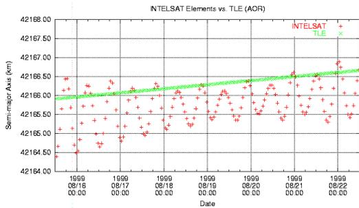
**Fig. 9.** Comparisons of semi-major axis between TLE and INTELSAT orbits.
