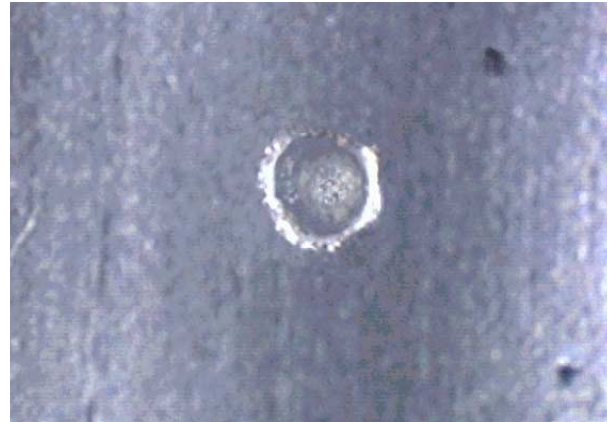
Fig. 5. Crater (0.8mm dia. by 0.47mm deep) in the 0.9mm thick aluminum line. SEM/EDXA revealed the impactor was a steel debris particle
