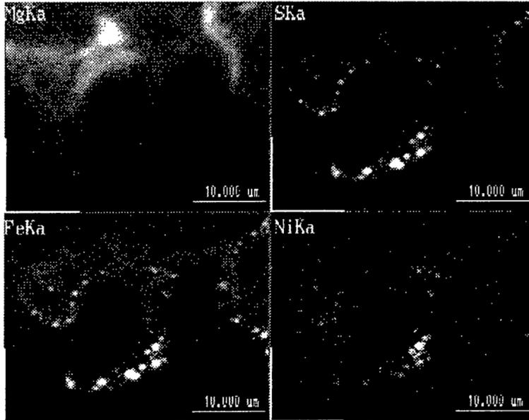
Figure 5. X-ray maps identifying the different elemental components within the residue.
