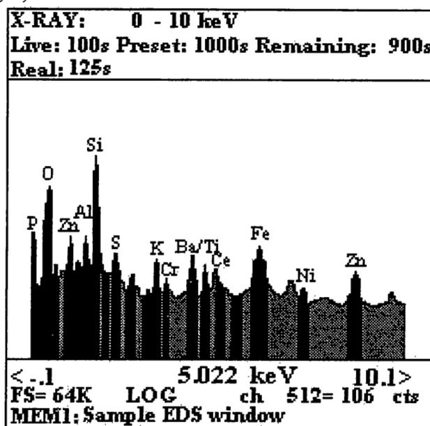
Figure 2. An example of the ED spectral windows used for X-ray mapping.
