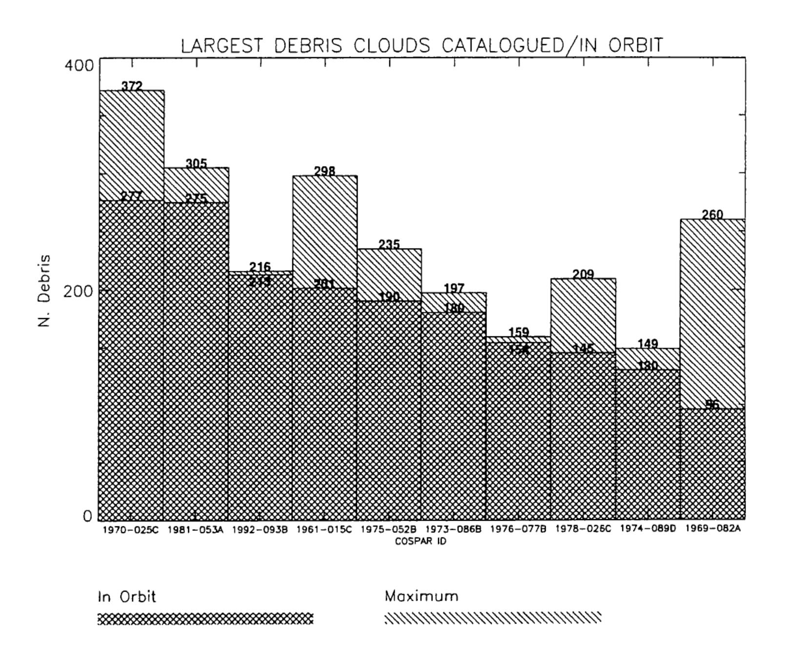
Figure 2: Maximum and current number of catalogued debris of 10 most severe fragmentations events.
