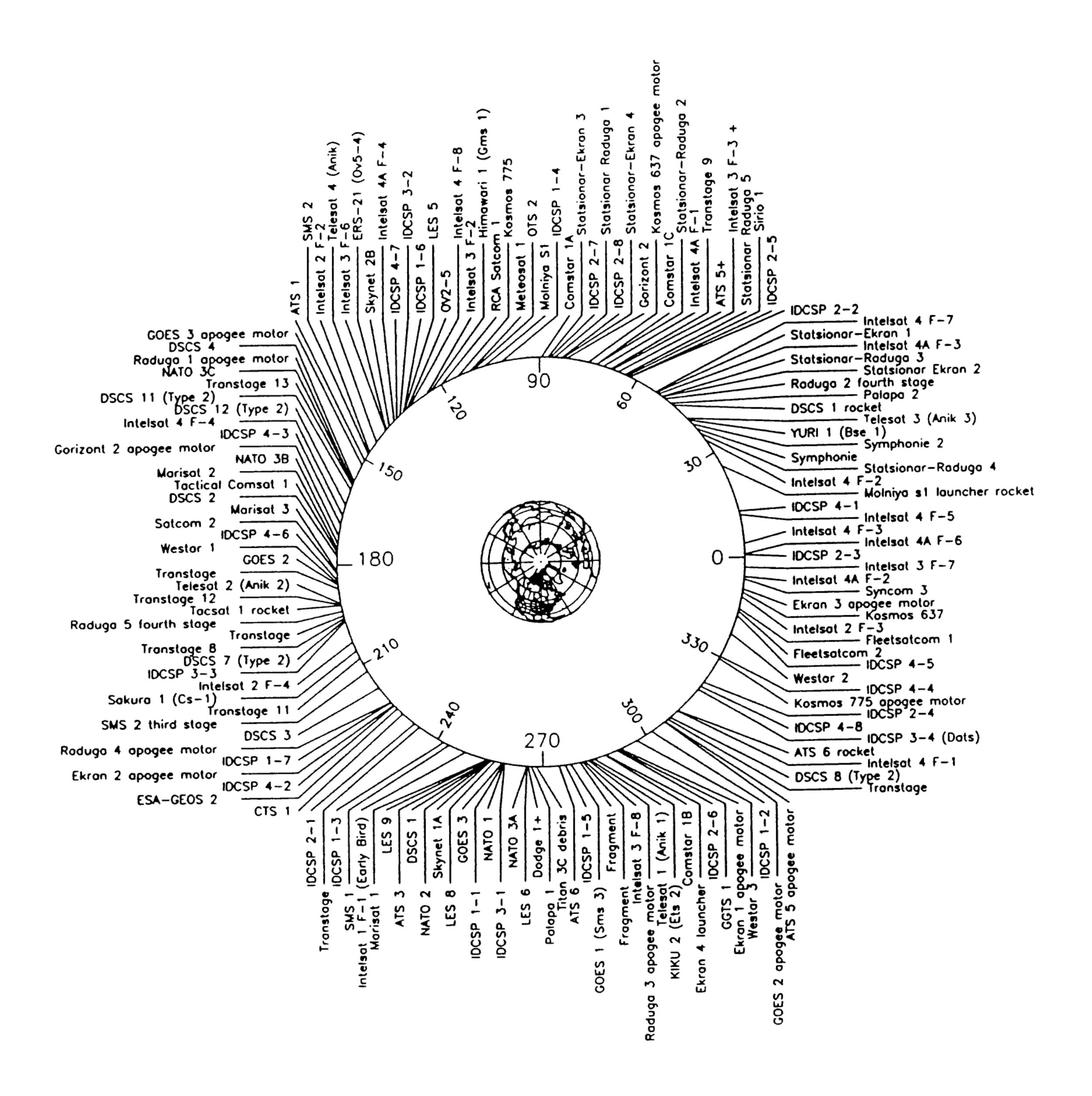
Figure 1: Geographical Longitude of near-GEO objects according to the last available orbit information (COSPAR Ids through 1979-087C)
