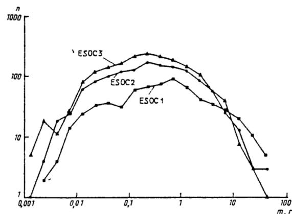
Figure 4. Number of fragments versus mass: ESOC experiments [1].
