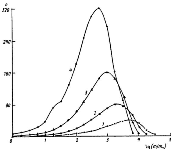
Figure 3. Number of fragments versus mass ( $\Lambda = 0.8$ ): 1 -  $s_* = 4000s_1$ ,  $N_{\Sigma} = 231$ ; 2 -  $s_* = 2000s_1$ ,  $N_{\Sigma} = 473$ ; 3 -  $s_* = 1000s_1$ ,  $N_{\Sigma} = 955$ ; 4 -  $s_* = 500s_1$ ,  $N_{\Sigma} = 1921$ .
