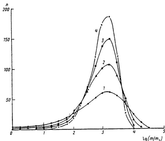
Figure 2. Number of fragments versus mass ( $s_* = 1500s_1$ ): 1 -  $\Lambda = 0.6$ ,  $N_{\Sigma} = 475$ ; 2 -  $\Lambda = 0.8$ ,  $N_{\Sigma} = 635$ ; 3 -  $\Lambda = 1$ ,  $N_{\Sigma} = 719$ ; 4 -  $\Lambda = 1.2$ ,  $N_{\Sigma} = 768$ .
