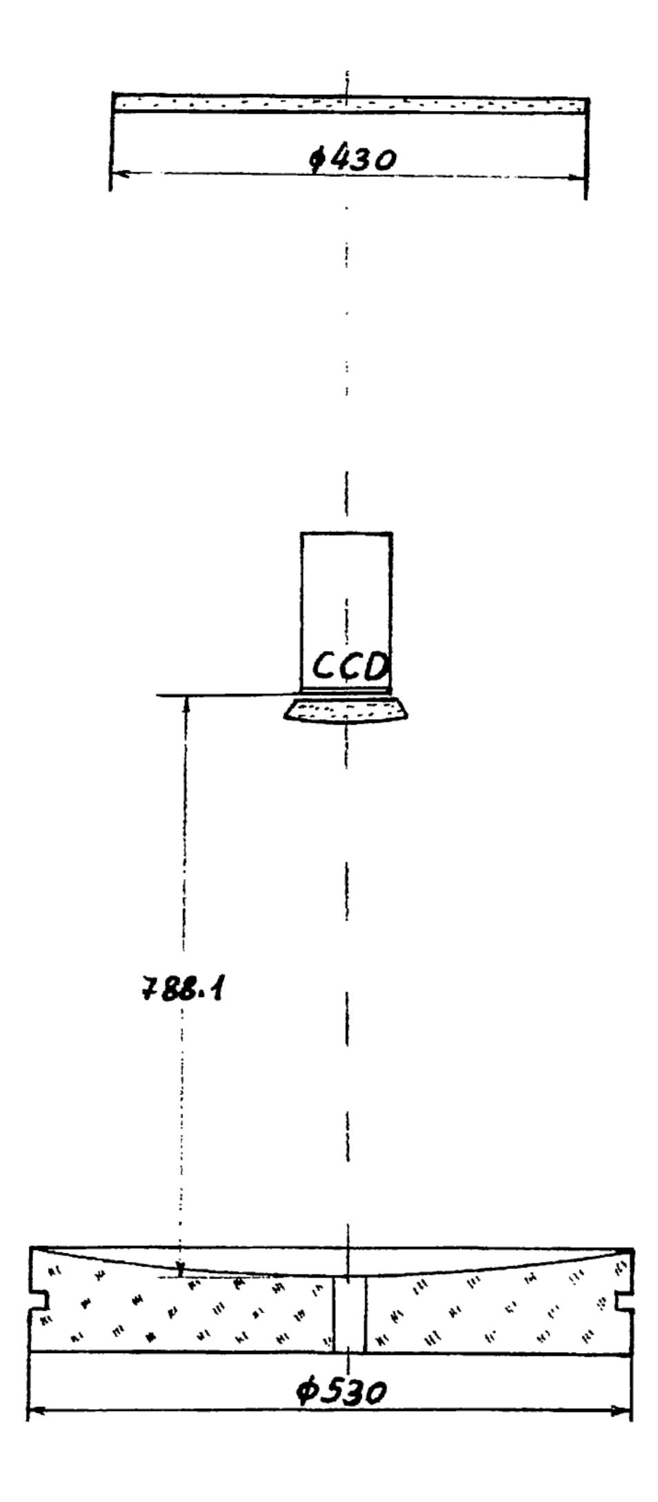
Fig. 1. The Schmidt optical system of SBG camera
