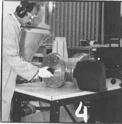
Fig. 6: W. Ockels testing repair methods with the cross-flanged test setup
