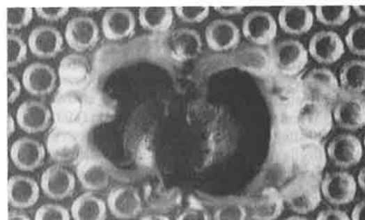
Figure 4. SEM Image and EDX Spectrum of Largest STS-50 Radiator Tape Impact
