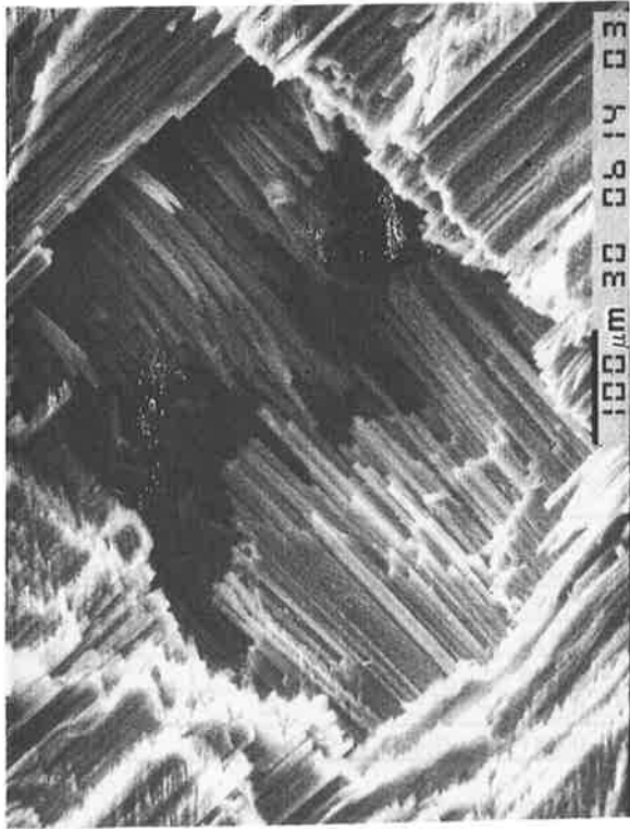
View of front face impact hole (x100)
