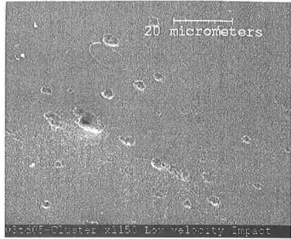
Figure 5. Crater cluster of top Al 1.5 \mu m foil with molten Silicon "pancake" splash.
