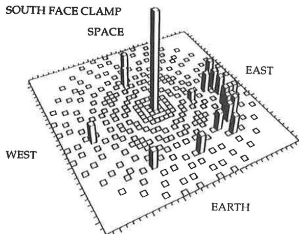
Figure 7. Plot of the elliptical craters on the South pointing clamp on LDEF. The "earth direction" impacts on the from particles in elliptical orbit with a southern perigee bias are seen. At the centre, the unresolved circular impacts are shown.
