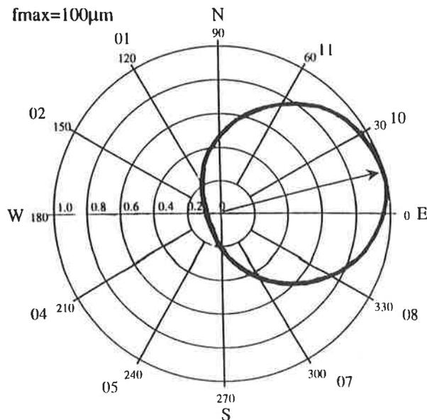
Figure 4 and 5. Angular distribution of the penetration flux for  $f_{\max} = 10$  microns (left) and  $f_{\max} = 100$  microns (right). The modest East to West ratio of the larger particles is seen, characteristic of a flux dominated by natural particulates, but in contrast to the space debris "signature" seen on the left at 10 microns.
