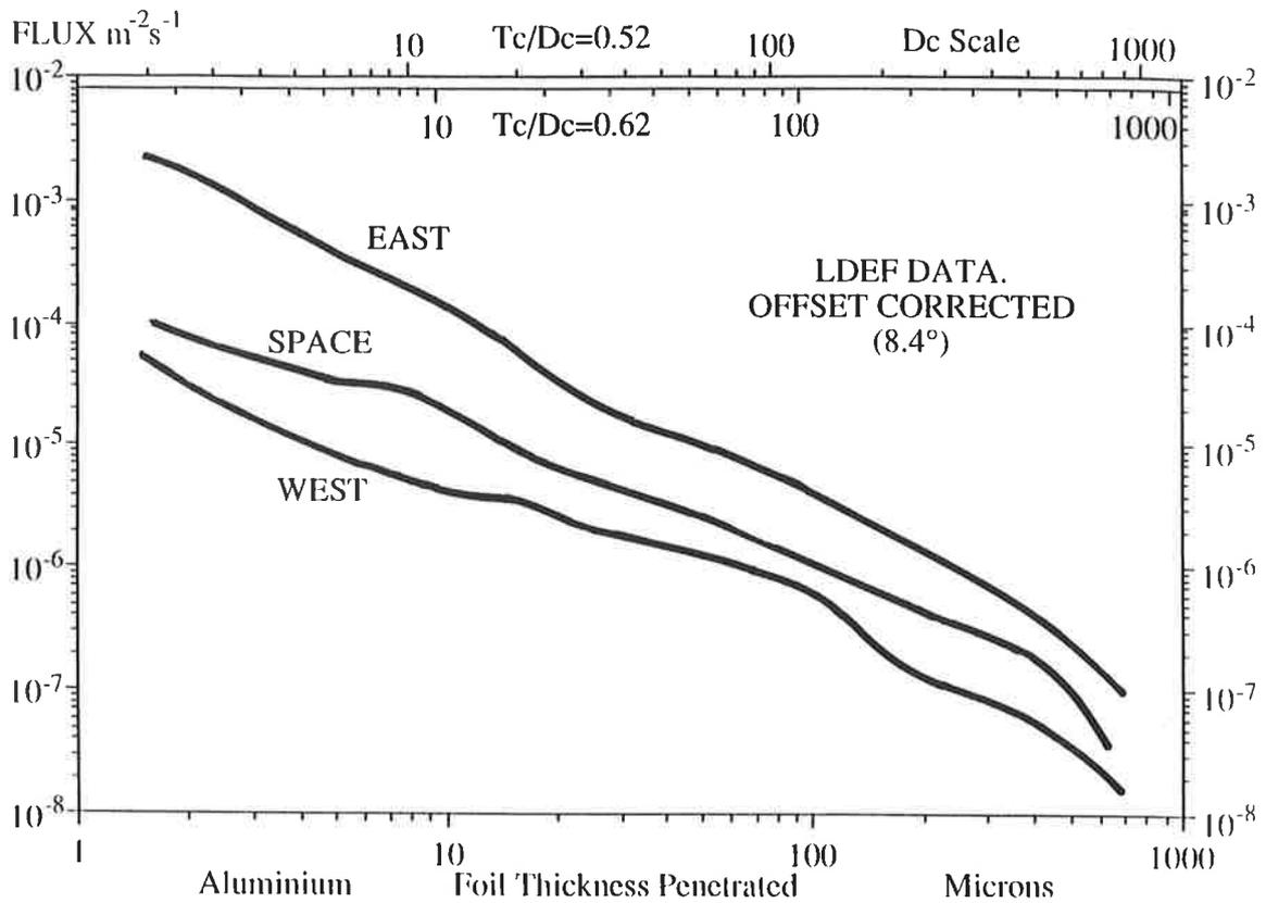
Figure 1. Flux distributions derived from the LDEF data set for aluminium shown for the East (ram) and West (wake) directions of orbital motion after correction for LDEF's offset. The space pointing flux is also shown.
