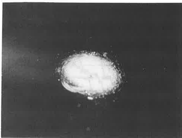
Figure 3. Recent impact damage to Shuttle window.
