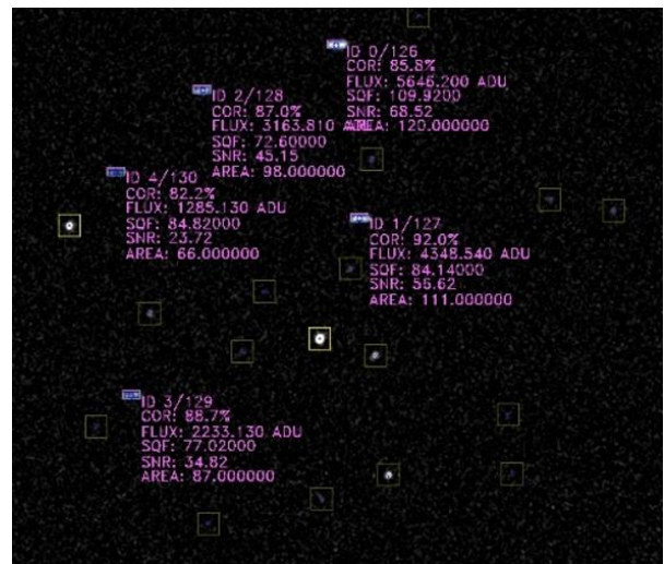
Figure 4: Example of detections on survey images. Stars appear as point-like (yellow) and satellites appear as streaks (purple).
