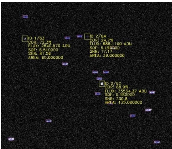
Figure 3: Example of detections on a satellite-tacking images. Stars appear as streaks (purple) and satellites appear as point-like (yellow).
