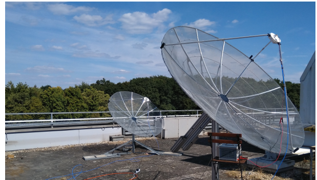
Figure 7. Reference System. The system consists of (currently) two parabolic antennas for the investigation of new synchronization techniques.
