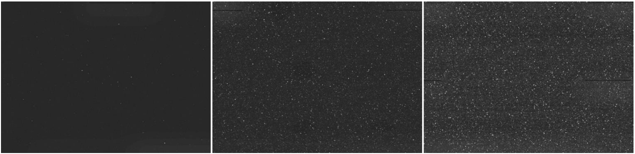
Figure 2. Empty field of view of 2s, 10s and 30s exposures showing the increase in hot pixels with the increase in exposure time. The hot pixels can change location on short timescales making them difficult to remove using automated algorithms.
